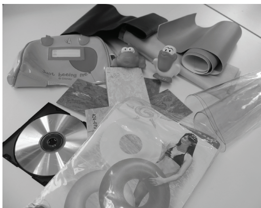
Figure 4. Plastic products (from paper I) which caused toxic leachates, i.e.: artificial leathers (brand S, G and M), children's handbag, bath tub squirt toys, floor material, table cloth (transparent), and inflatable bathing ring. The CD was only toxic when cut into pieces and the silver layer was exposed [1].
