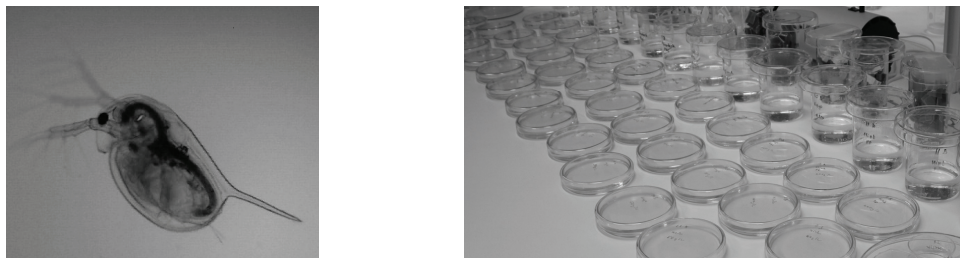
Figure 3. Test organism Daphnia magna (size: 0.8 mm newborn, 5-6 mm adult), and Petri dishes during toxicity tests.
